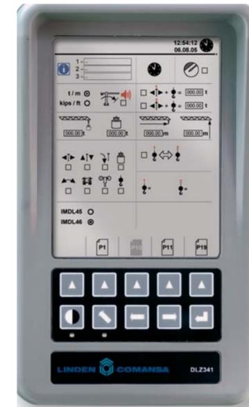
The new LINCOMATIC system has been designed and developed in cooperation with Linden Comansa and the leader in dedicated Electronic Control Systems, SMIE. This system makes available the information the crane operator needs to noticeably improve his crane operation and control experience: ranges, hook height, moment, maximum liftable load, register of the latest cycles carried out, etc.
